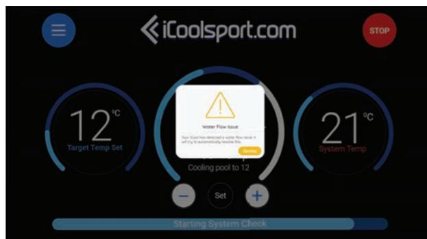
It can occur if air is trapped in the water pipes or in the pump, or if flow is restricted in the hoses by some sort of blockage. There could be an air leak in the hoses or pipes from the pool or trapped air in the system.
