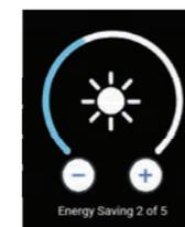
You can set different levels of energy saving. Level 1 provides full cooling power, Level 5 saves the most electricity. We recommend keeping it at 2 as a default.
