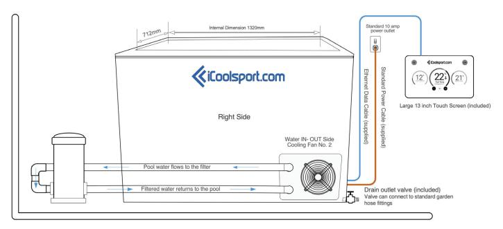
Filter System can be mounted in any convenient place near the pool, or in an adjacent room or outdoor space within 15-20 meters maximum distance.
