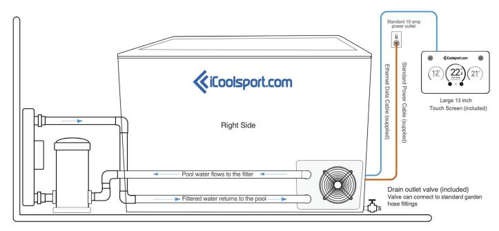
Filter System and Ultra Violet Antibacterial System can be mounted in any convenient place near the pool, or in an adjacent room or outdoor space within 15-20 meters maximum distance.
