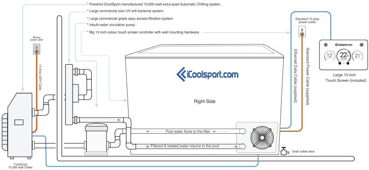
Data cable to the external chiller can be routed wherever convenient. Maximum length 30 meters
